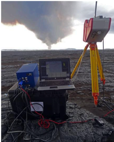
Figure 2: Envicam-2 UV (blue) and NicAir-2 IR camera (on tripod), monitoring emissions from Bardarbunga volcano, Iceland.
